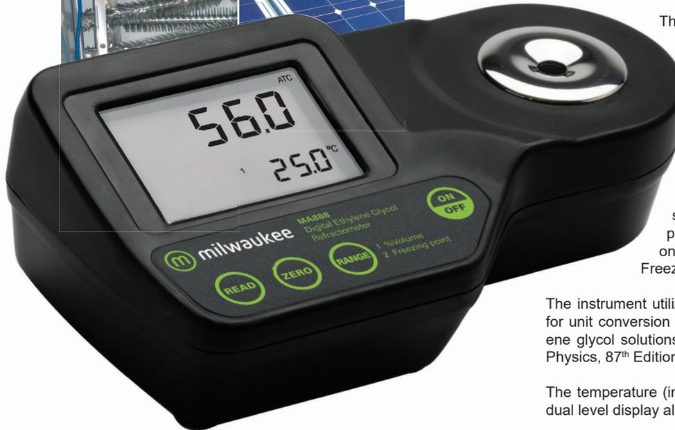
The MA888 is an optical instrument that employs the measurement of the refractive index to determine the % volume and freezing point of ethylene glycol based coolants or antifreeze.
