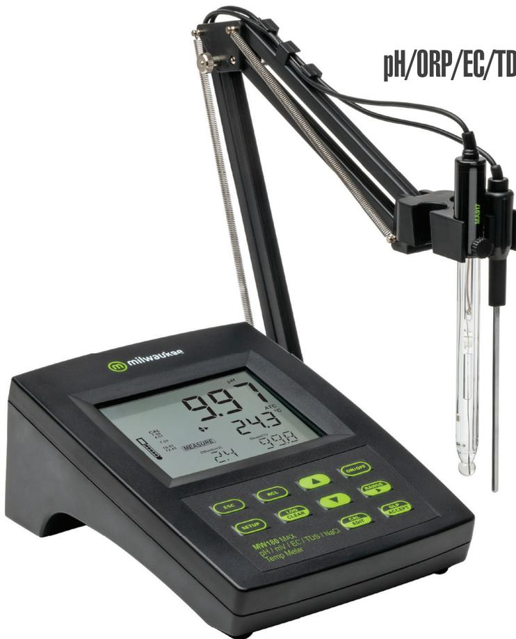
**MW180 MAX** is a compact and versatile bench meter with a user-friendly interface that can measure six different parameters – pH, ORP, EC, TDS (Total Dissolved Solids), percentage of salinity (NaCl%) and temperature – when paired with the respective probe.
